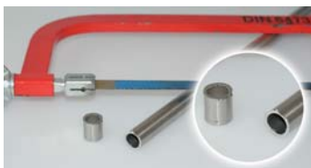
Result with a hacksaw (inside and outside burr)
