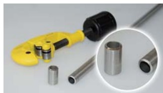
Result tube cutter (inside burr)
